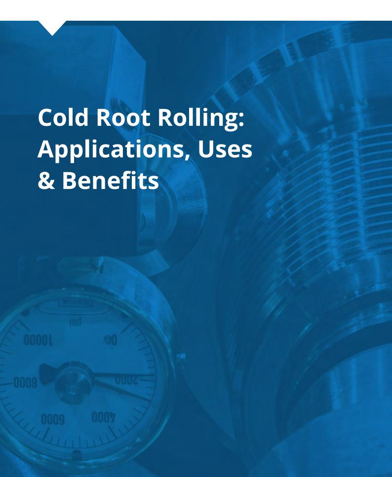
Cold root rolling is a useful process by which the root of a threaded pipe connection is strengthened, thereby reducing the risk of pipe failure—especially in pipes that experience constant use, high pressures, and exposure to corrosive materials. Cold root rolling has proven to be an effective preventive technique that can save companies significant time and money.
