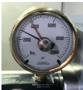
Gage needs pre-load adjusted down slightly
