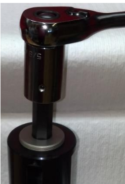
Pre-load being adjusted
