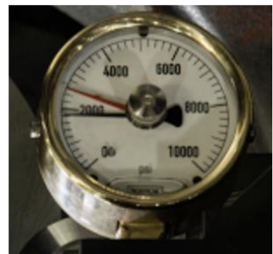
Pre-load set correctly, less than 1000 psi apart
