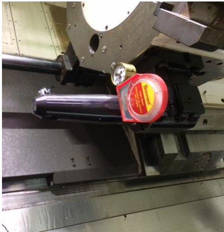
Level used on slant bed lathe
